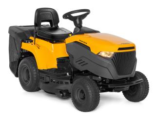
STIGA engine with net power output of 5.8 kW @ 2400 rpm
