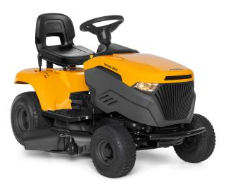
STIGA engine with net power output of 6.5 kW @ 2800 rpm
